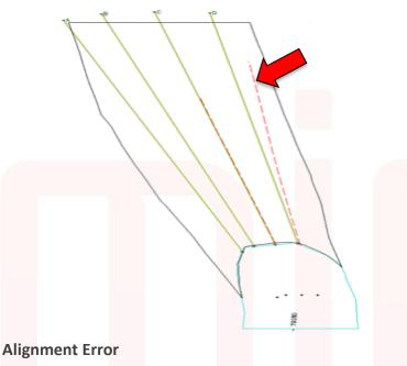
If the alignment of a blast-hole is incorrect at the collar of the hole, the error will increase proportional to the length of the blast-hole.
