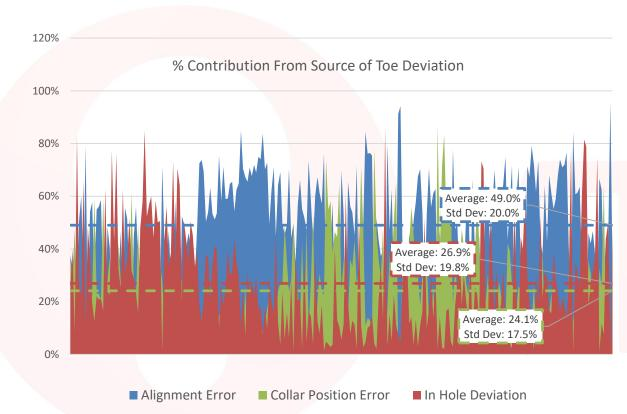
A series of downhole survey results and survey collar pick-ups from a number of sites were analysed to determine what proportion of alignment error, collar error and in-hole deviation contributed to overall blast-hole deviation.
