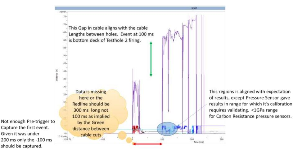
This is too short a gap for Testhole 1 to have been timed incorrectly – top down. If it was the gap should have been 400-100 ms >> 300 ms
