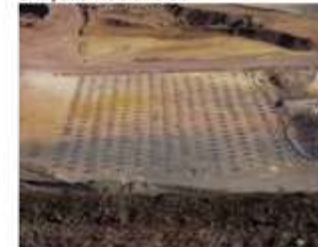
Drill pattern on a bench
